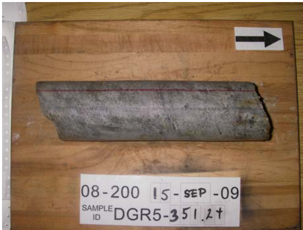
Salina Formation A2 Unit Evaporite – Anhydritic Dolostone DGR-5, CR049
