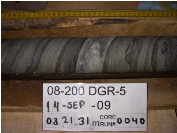
Salina Formation A2 Unit Carbonate – Anhydritic Dolostone DGR-5, CR040
