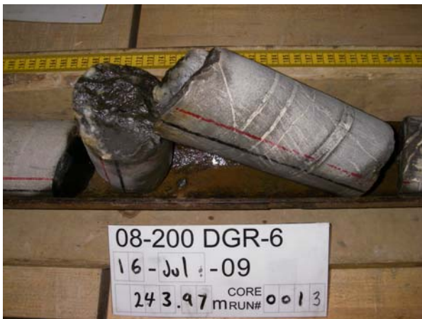
Salina Formation F Unit – Dolostone with Anhydrite/Gypsum veins DGR-6, CR013
