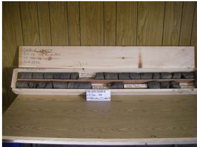
Salina Formation A2 Unit Carbonate – Dolostone DGR-6, CR057
