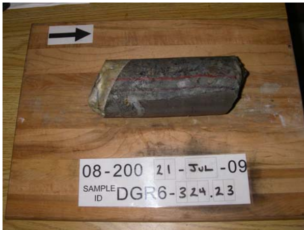
Salina Formation B Unit – Brecciated Dolomitic Shale DGR-6, CR039
