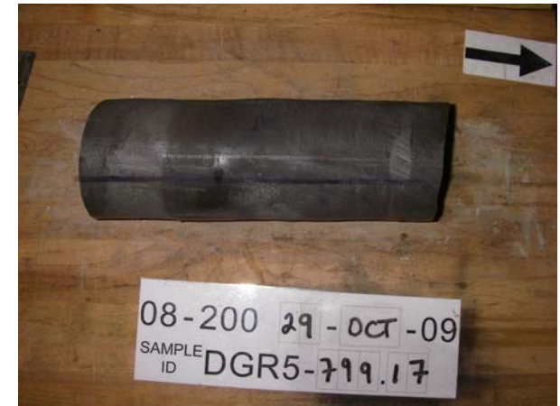
Kirkfield Formation – Interbedded Argillaceous Limestone and Shale DGR-5, CR200
