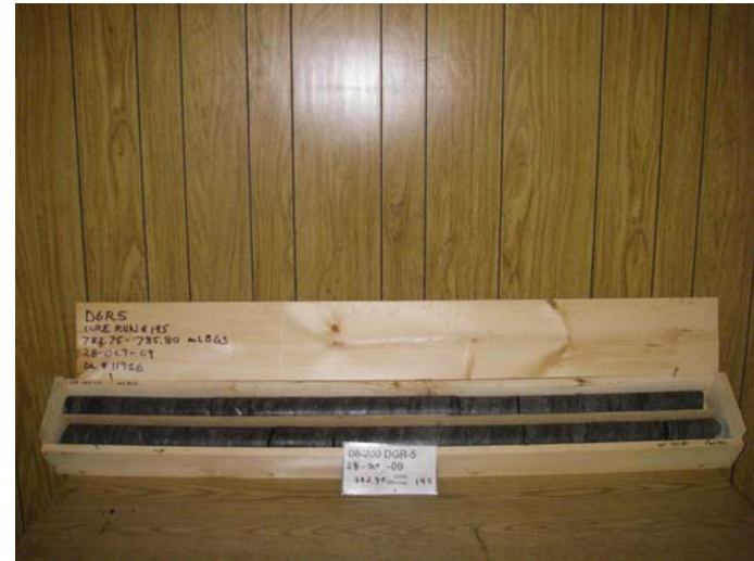
Kirkfield Formation – Interbedded Argillaceous Limestone and Shale DGR-5, CR195
